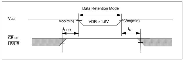
Note: Full device operation requires linear Vcc ramp from VDR to Vcc(min) > 100  $\mu s$
